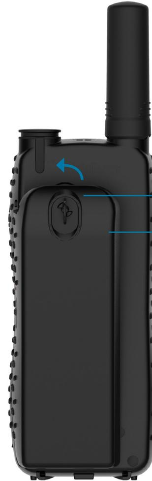
1. Lift D-ring up and rotate counterclockwise 90 degrees
